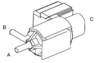
When the valve is OFF, A is closed off the actuator B is vented to atmosphere C When the valve is ON, the solenoid connects the actuator B to the vacuum box A
